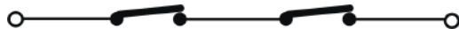
Connection of two N.C. contacts in series (e.g. Photocells, Stop, Edge, etc.)
